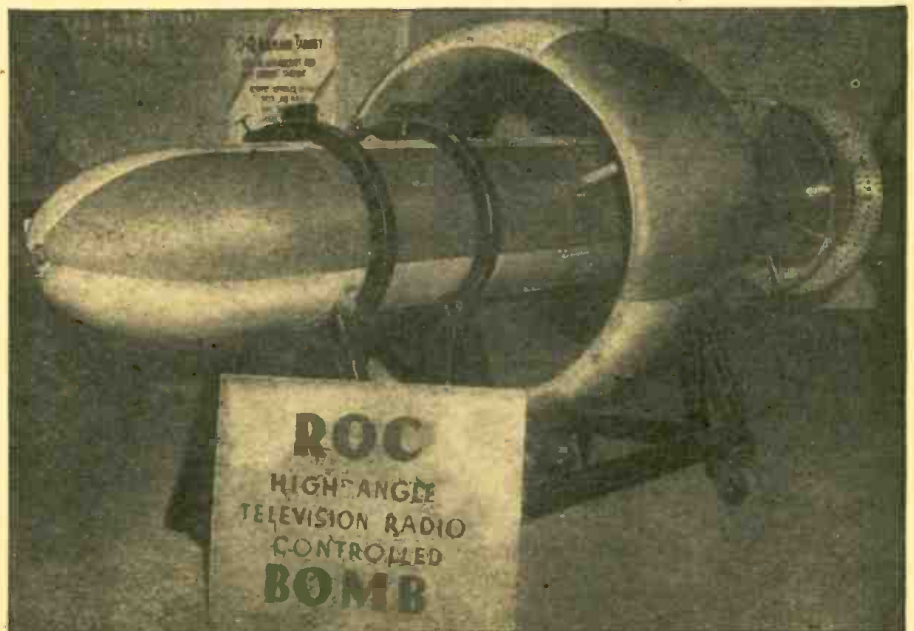
The Roc televises a view of the target back to its control, who guides it accordingly.
